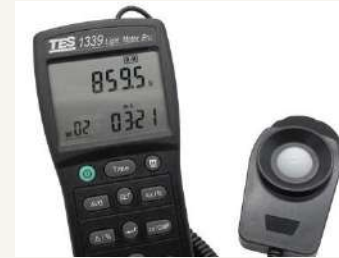
TES-1339 Professional-grade illuminance meter Four-digit dual-display LCD with clear viewing function. Spectral response is less than 6%. Measurement range is from 0.01 Lux to 999,900.
