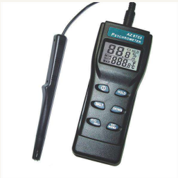
AZ8723 HVAC Humidity Meter & Probe
