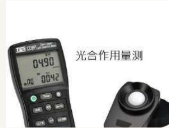
TES-1339P Photosynthesis measurement - illuminance photometer Photosynthetic photon flux density (PPFD) (micro; mole/m 2 )
