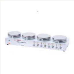
H05-1 Constant temperature magnetic stirrer - four positions - strong magnetic force - temperature control
