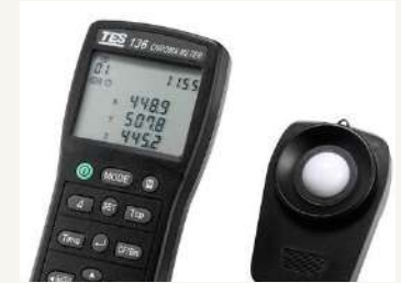
TES-136 Color temperature colorimeter Three groups of 4-digit display LCDs
