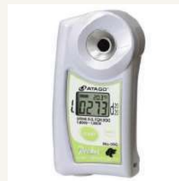
PAL-DOG Dog urine specific gravity refractometer (S.G.)
