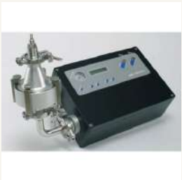
MAS-100 CG Ex Compressed Gas Microbial Sampler
